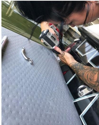
Drill 1/8" holes, lightly countersink
